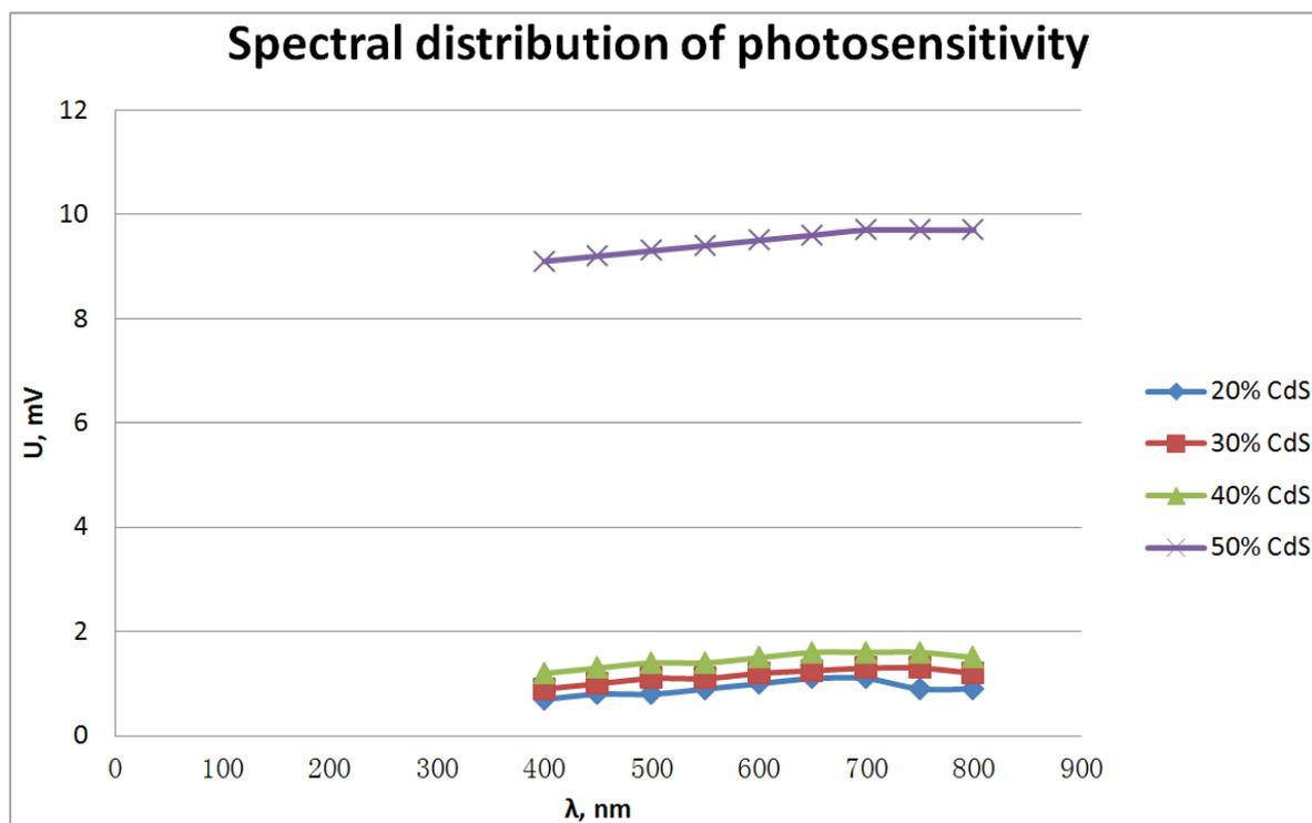
**Figure 3.** Spectral distribution of photosensitivity of High-density polyethylene and CdS containing samples: × -50% CdS +50% polyethylene; ▲ - 40% CdS +60% polyethylene; ■ - 30% CdS +70% polyethylene; ◆ - 20% CdS +80% polyethylene.
